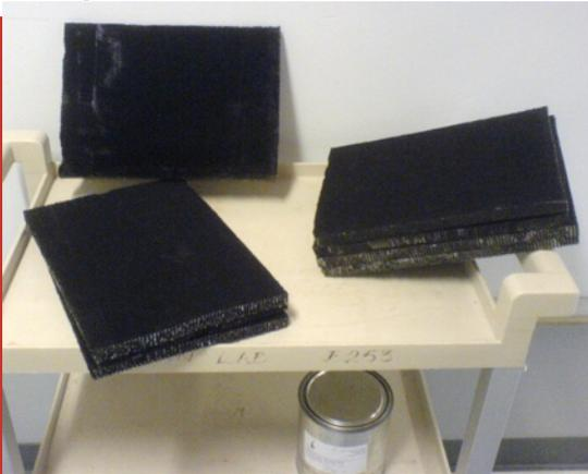
You will find that it is easy to slide the twelve pieces of cut catalyst into the room air filter, leaving you with a self-contained rolling ozone recirculating catalyst unit.
