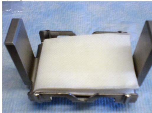
In either case, you will first fold some paper towels to fit each tray. Then when all is ready, quickly transfer your slide rack from the final wash into the centrifuge bucket. Place in centrifuge.
