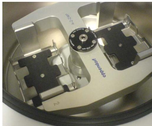
Close centrifuge, press "start" button, watch speed display, it will start up and reach 70rcf in a while. After 5 min. it will slow down, and it will beep when done.
