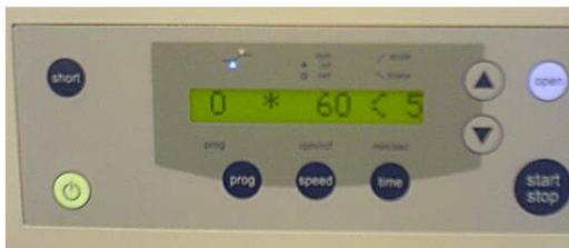
Press Speed button until it shows a \* and a number. When Speed shows something like \*70 that means 70 RCF which is the same as 70g. If it does not show \*70 then press Speed until it shows \*something and then use the up and down arrows to make the number \*70.
