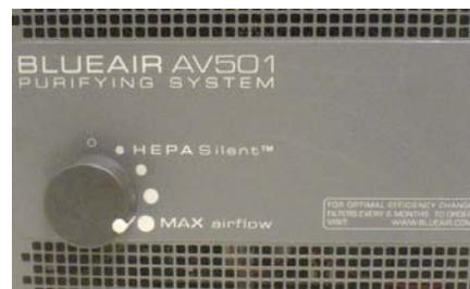
ozone free room. While you are there, find the BlueAir Purifying System with ozone catalyst and rotate the switch to **MAX airflow**.
